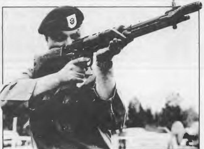
Special Forces sergeant with a German FG-42 assault rifle in shoulder firing position. This WW II era weapon broke new ground in small arms design. It fired its 7.92mm rounds from a closed bolt in semiauto mode, and from an open bolt in full auto mode. Photo from "Special Forces Combat Firing Techniques."
